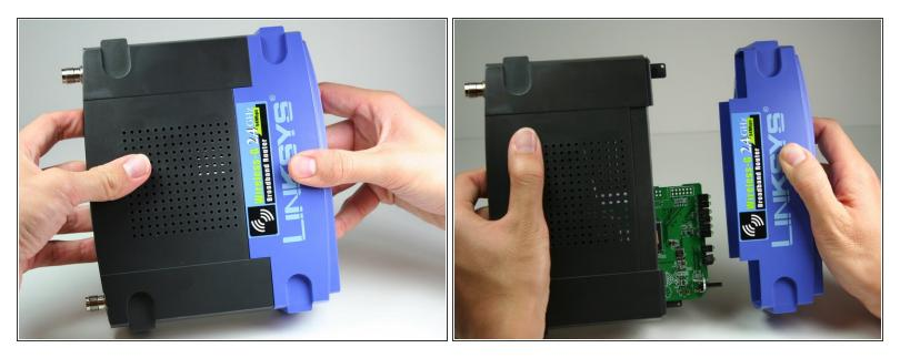
• Using a bit of force, remove the blue plastic case.
