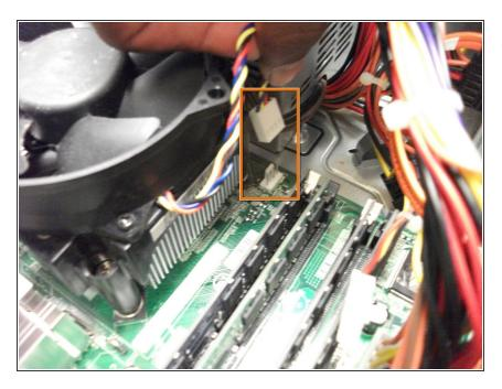
Remove the fan's power cable from the motherboard.
