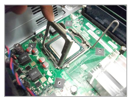
Open the metal casing over the processor.
