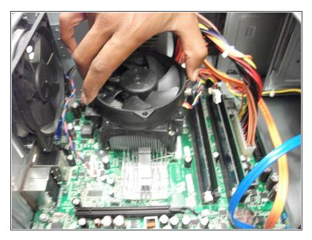
Remove the fan and heat sink.
