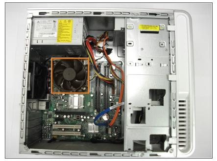
Locate the processor's heat sink and fan.
