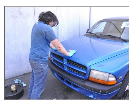
Gently lower the hood until it clicks into the secondary latch, then press firmly on the top of the hood until it locks into the main latch.
