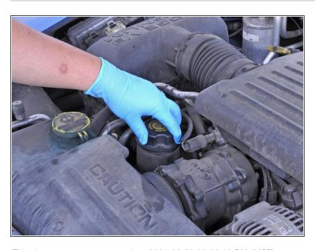
Place the oil filler back over the oil filler hole and turn it clockwise by hand until it is snug.
