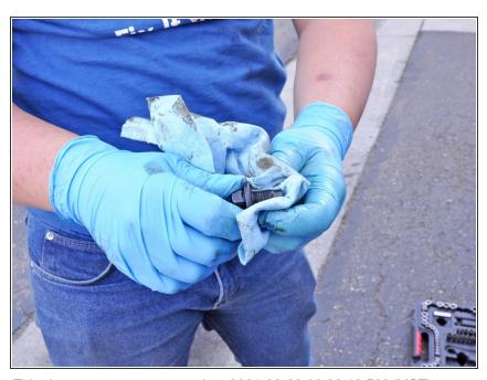
Wipe off the oil drain plug using a clean towel or rag.
