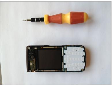
Using T6 Torx screwdriver remove the six 15 mm torx screws.
