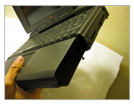
The battery compartment is located in the front-right side of the laptop.
