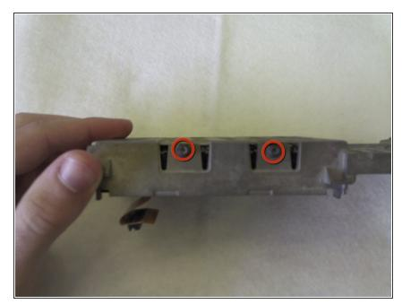
In order to remove the hard drive, remove the four .22 in. screws circled in red found on both sides of the metal chassis with a Torx #9 screwdriver.
