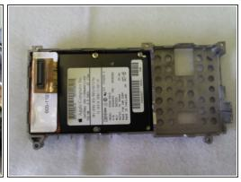
Remove the metal chasis that holds the hard drive.
