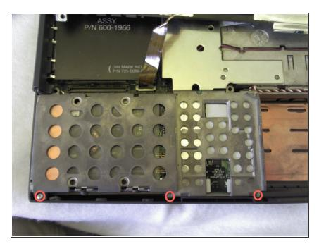
With a Torx #9 screwdriver, remove the three .30 in. screws that hold the metal frame in place.
