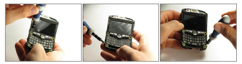
• Use a T6 Torx screwdriver to remove the four screws located on the corners of the keyboard frame.
