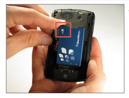
• Pull up on the top edge of the battery to remove it.
