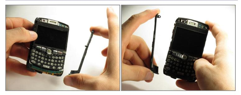
• After the bottom two screws have been removed the side casings can be removed.
