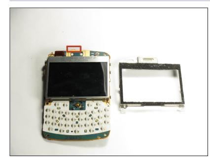
(*i*) Place the motherboard on a flat surface with the LCD screen face up.
