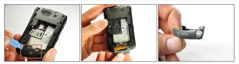
• Use a plastic opening tool to gently pry the bottom cover loose.
