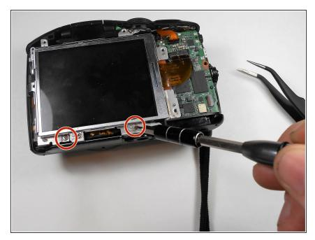
Remove the two 2mm screws from the bottom of the screen with the size J000 screw driver.
