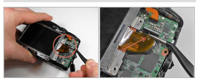
• Use the tweezers to carefully detach the screen's flex ribbon from the circuit board.
