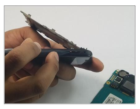
Remove the desired button by pushing inward with the spudger or disconnecting the rubber pin connections.
