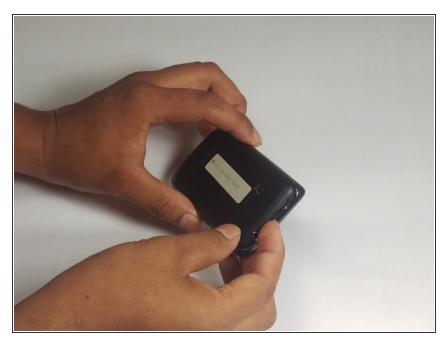
Using your hands, carefully remove the back panel by popping the open slit, near the headphone jack, outwards.
