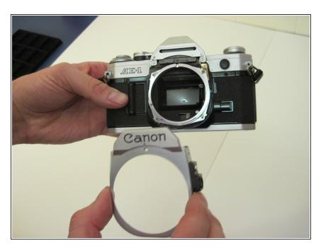
Remove the lens casing by pulling it away from the body of the camera.
