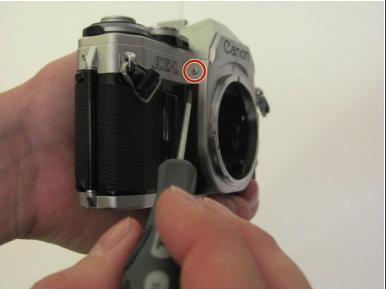
Remove the remaining two screws from the right and left sides of the lens outer casing using a Phillips #00 screwdriver.
