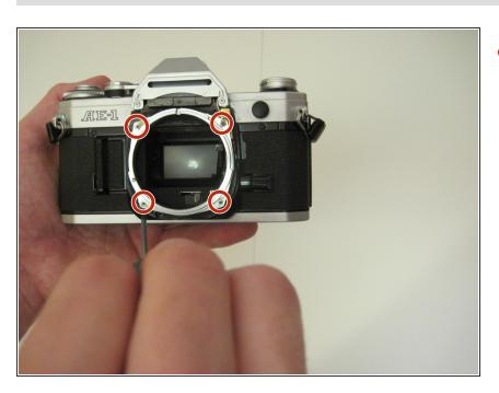
Remove the four #00 screws from the SLR lens mount using a Phillips #00 screwdriver.
