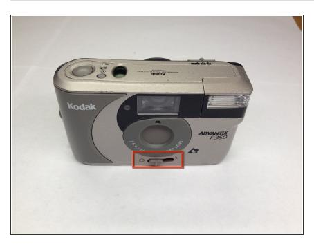
Turn off camera by moving the highlighted switch to the O-Position.
