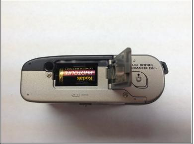
To open the cover of the battery slot, push the highlighted tab in the direction of the arrow next to it, and gently lift.
