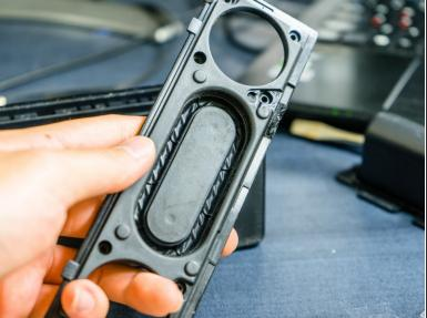
• Two passive radiators are present inside the device. They're fairly heavy but rubberized, and they resonate and are tuned for low frequency reproduction. These move a LOT when it's playing. 7-10mm per side.
