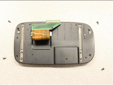
Use the T5 Torx screwdriver to remove four 5mm screws that secure the back of the screen casing.
