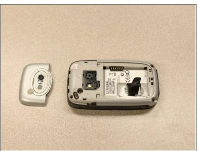
Work the <u>spudger</u> around the edges of the camera cover until it comes off.
