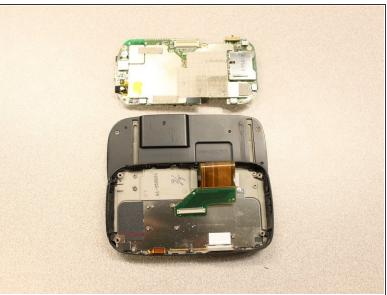
Remove the flexible connection from the motherboard.
