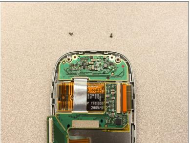
Unscrew the two 3mm phillips #0 screws from the bottom of the device that secure the rigid flex board to the screen panel.
