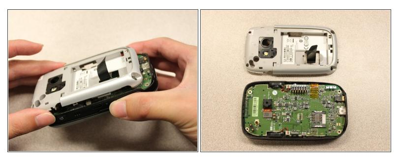
• Once all the clips are open, remove the inner panel from the phone.
