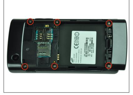
Remove the six 4.5mm #000 Phillips screws.
