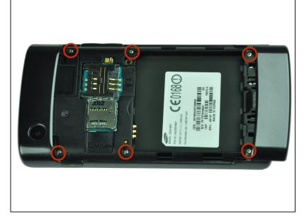
Remove the six 4.5mm #000 Phillips screws.
