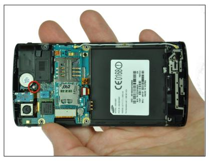
Use the Phillips 00 screwdriver to remove the single screw holding the speaker assembly to the LCD.
