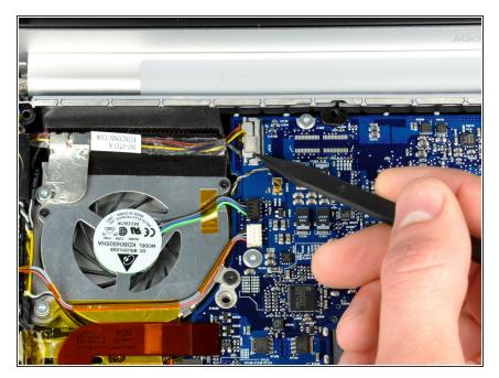
Use a spudger to disconnect the iSight cable from the logic board by sliding the cable to the left and out of its connector.
