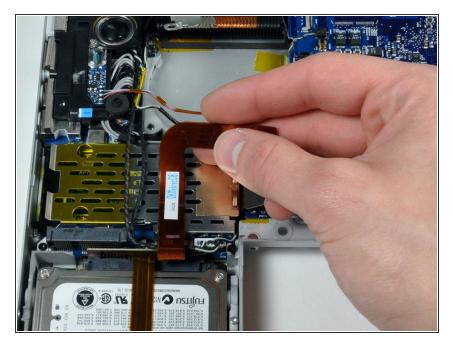
Peel up the orange hard drive cable from above the ExpressCard cage.
