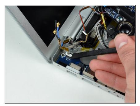
Use a spudger to disconnect the inverter cable from the corner of the left I/O board.
