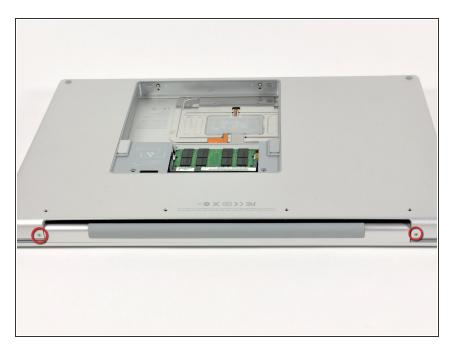
Rotate the computer 90 degrees and remove the two 3.2 mm Phillips screws from the rear of the computer.
