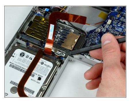
Use a spudger to disconnect the speaker cable from the corner of the left I/O board.
