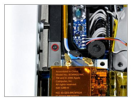
Remove the single black T6 Torx screw located just above the Airport Extreme card.
