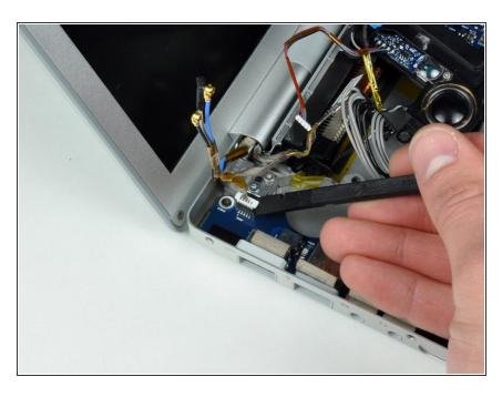
Use a spudger to disconnect the inverter cable from the corner of the left I/O board.
