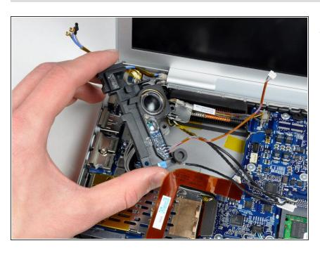
Lift the left speaker assembly out of its housing and place it in the area previously occupied by the left fan.
