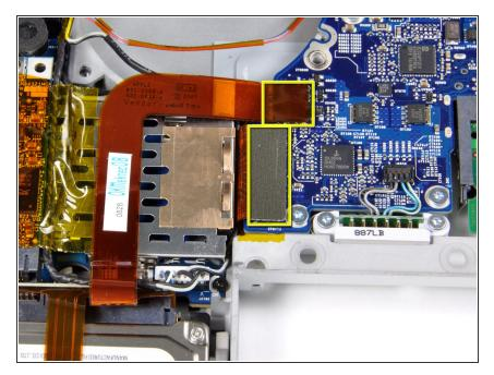
Disconnect the hard drive and ExpressCard connectors from the left side of the logic board.
