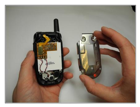
Remove the metal cover by lifting up and away from the device.
