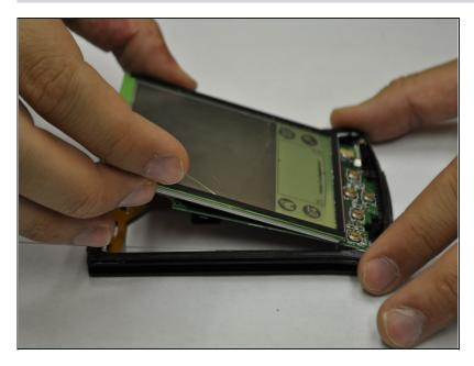
• Remove the screen from the plastic casing.
