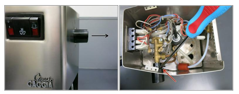
• Pull the steam knob out. If its too hard, try to gently pry it out with a flathead screwdriver from the inner side of the machine.
