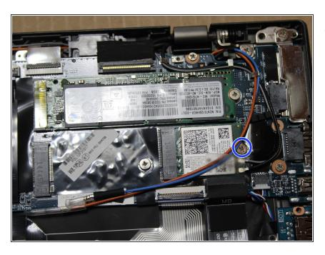
Remove screw holding the wireless card in place.
