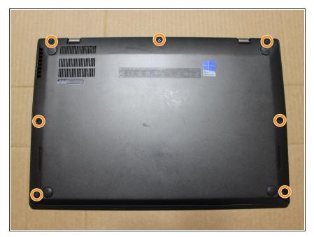
Using the #0 Phillips screwdriver, loosen the seven cover screws. they will not come all of the way out.
