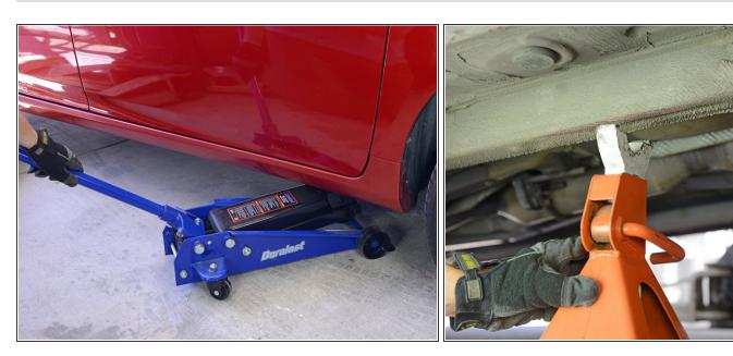
When you've finished servicing your vehicle, use the jack to raise it back up an inch or so, and remove the jack stand(s).
