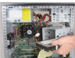
• Fully remove the hard drive cage by sliding it towards the back of the device and pulling down.
