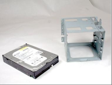
Remove the hard drive from the hard drive cage by pulling it outward from the cage.
