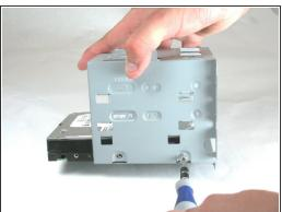
Remove the two Torx T15 screws holding this side of the hard drive in place.
