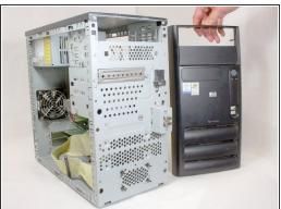
Remove the front bezel by pulling upwards and out from below the lowest air vent.
