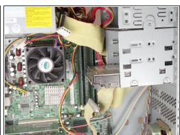
Remove the IDE data and power cables from the hard drive.
