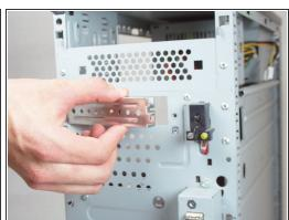
Remove the external drive faceplate by removing the two Torx T15 screws.
