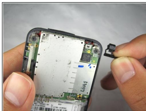
**i** While removing the back cover do not lose the power button. It is held in place by the back cover and may fall off during removal.
