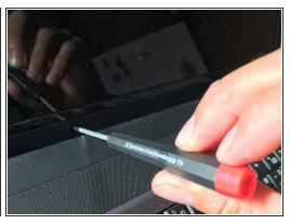
Remove the 8 pads and the underlying screws
