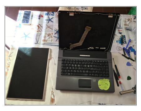
Remove the LCD panel and replace with the new one
