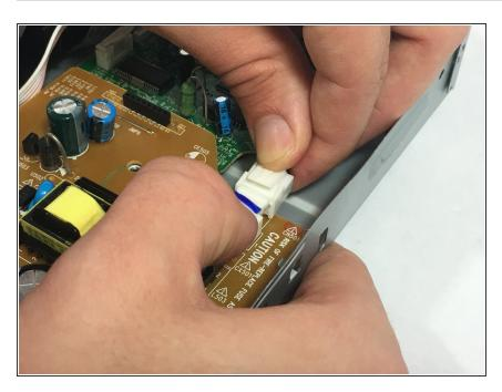
Disconnect the white power cord connector from the motherboard.
