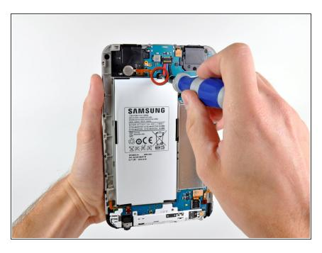
Remove the single Phillips screw securing the battery to the motherboard.
