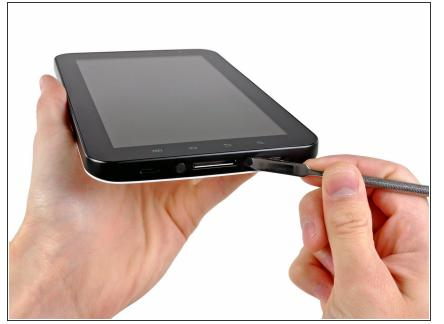
• Use the flat end of a metal spudger to pry the two plastic tabs near the dock connector off the rear case.
