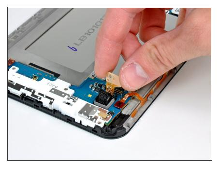
• Lift and remove the rear camera from the Galaxy Tab.
