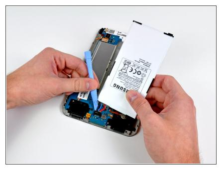
Use the edge of a plastic opening tool to pry the battery connector straight up off its socket on the motherboard.
