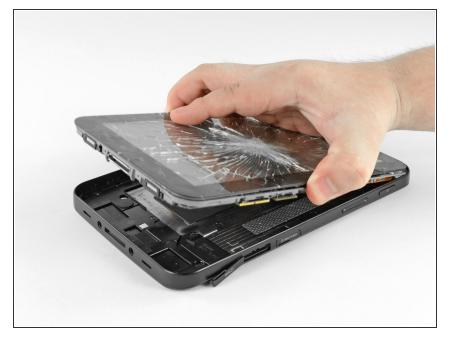
• Lift and remove the front panel assembly from the rear panel.
