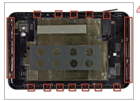
The following steps will require you to disengage several clips (highlighted in red) around the perimeter of the rear case. The clips are delicate and fragile; proceed with caution.
