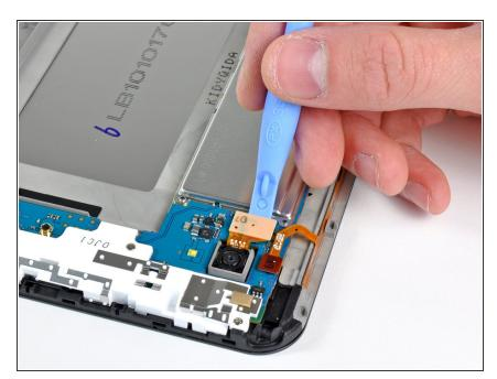
• Use the edge of a plastic opening tool to pry the rear camera connector up from its socket on the motherboard.
