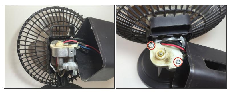
• Remove the 2 screws fastening the lid on the oscillation gear housing with a Flathead Screwdriver.
