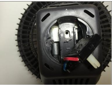
Remove the screw that holds the housing assembly in place by using a Phillips #2 Screwdriver.
