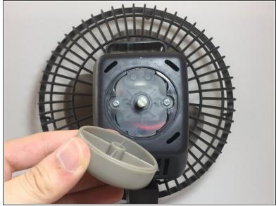
• The on/off and fan speed nob can be removed by simply pulling it away from the main housing.
