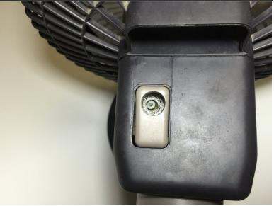
On the top of the fan, there is a screw fastening the oscillation button to the gear train within the housing. Remove this screw with the Phillips #0 Screwdriver.
