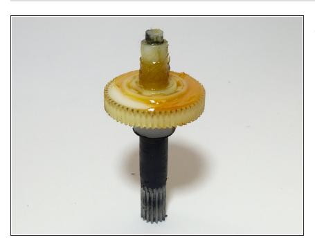
The oscillation gear has been removed and fresh grease can be applied or it can be replaced.
