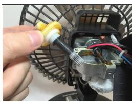
The oscillation gear is removed by pressing it up from the bottom.
