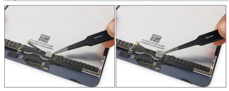
• Use tweezers to lift the home button control hardware module off the display assembly.
