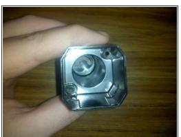
Slide the plunger tube guard reinforcement plate (from the Stage 1 kit) into the guard we removed in step 5.
