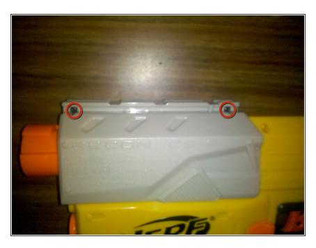
Now remove the two Phillips #0 screws on the cocking mechanism itself. They're the same size as all the other short screws.
