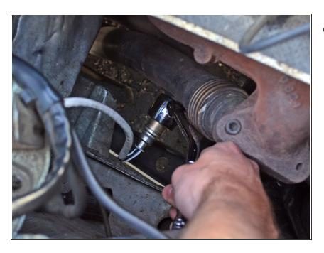
Use the oxygen sensor wrench to torque down the oxygen sensor.
