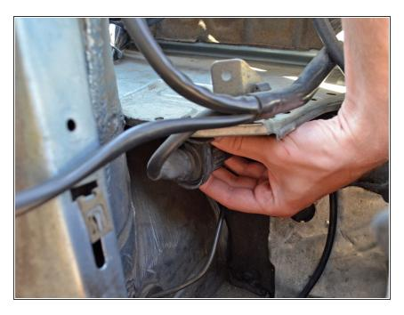
Unscrew the oxygen sensor connector (lefty, loosey) and unplug it from its socket leading to the engine harness.
