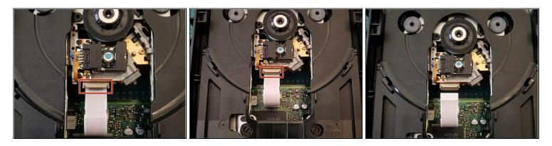
Gently press back on the ribbon retention tab and pull back on the ribbon cable
