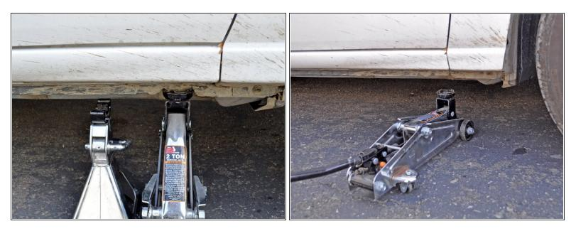
Make sure there is no one under the car before removing the jack stand and lowering the car!
