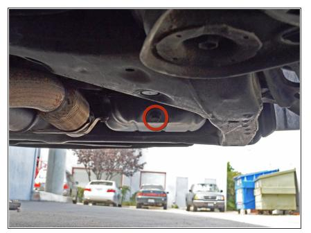
Locate the 14 mm hex oil drain plug. It will be on the passenger side of the car facing backwards.
