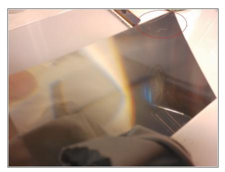
This is one of the polarizing layers. In the picture circled in red you can see why using a playing card or a tape-covered blade might be a good idea. The scratches didn't show really at all in the end, though.
