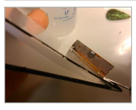
As you remove the layers, mind the LCD flex cable, as it is very fragile, and your knife can slip through it very easily, rendering the whole screen totally worthless.
