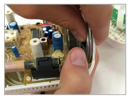
Locate the speaker and desolder the contact points.
