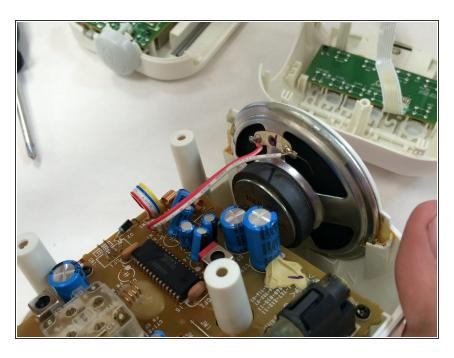
Place the new speaker in the slot and resolder the contact ports.
