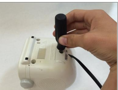
Unscrew the screws located here with a Phillips head screwdriver.
