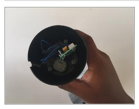
Step 9: Carefully lift the lid off of the sharpener.
