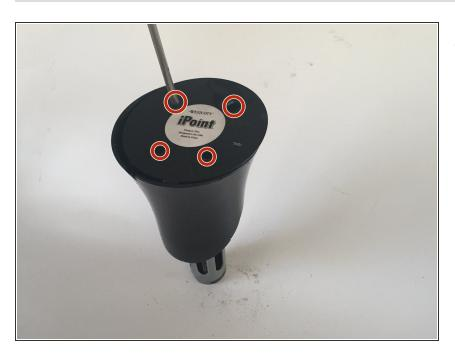
Step 7: Take a screwdriver and unscrew all of the screws on the bottom.
