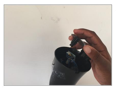
Step 8: After all the screws are removed gently take off the bottom of the sharpener.
