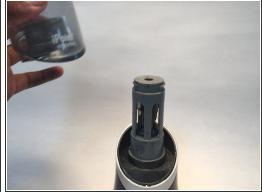
Step 4: Grab the center of the sharpener and lift it up to remove the piece.
