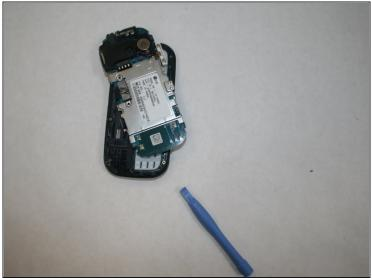
• Use a spudger or your finger to detach the motherboard from it's housing. Slowly pry along the edges to free it from the plastic grips that hold it in place.
