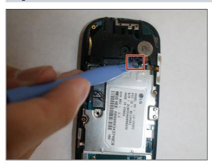
Use a spudger to detach the small red and blue cable from the motherboard. Do this by slowly lifting up each side until it pops out of it's housing.
