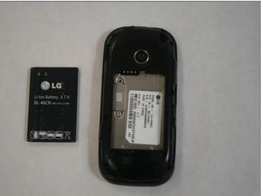
• Simply use the provided tab to lift the battery our of it's housing and set it aside.
