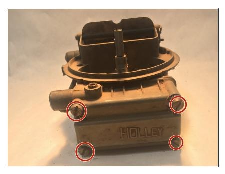
Remove the four 47 mm flat head screws.
