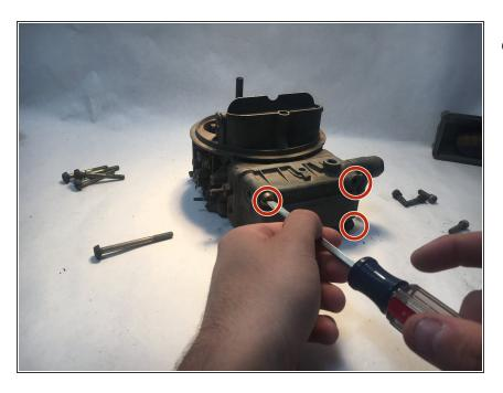
Remove the four 63 mm flat head screws.
