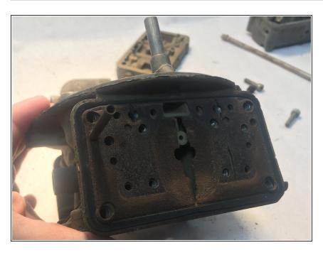
Using a flat head screwdriver, remove the thin gasket from the side of the carburetor.
