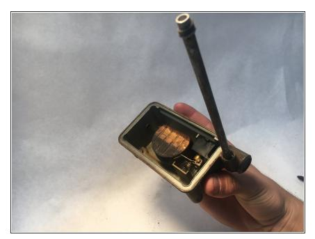
Remove the bowl and the steel fuel line from the side of the carburetor.
