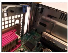
Unscrew the two screws holding the Motherboard down (annotated with the red circles).
