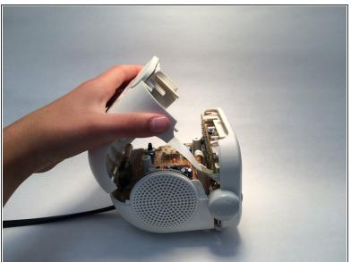
To open the top casing, pull it upward.
