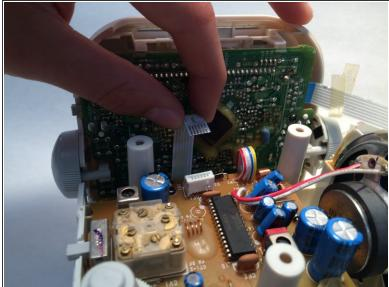
Pull upward on the blue and white ribbon cables to remove them. This will make it easier to remove the speaker.
