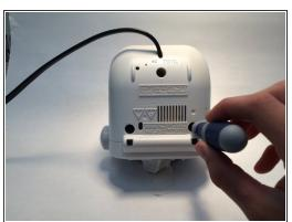
Detach the top of the plastic casing. Use a Phillips head screwdriver to unscrew the three bottom screws.
