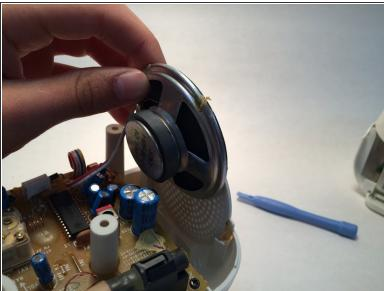
Pull the speaker upward to remove it.
