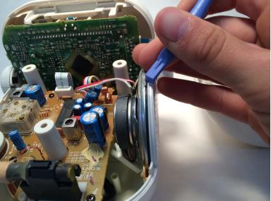
Use the plastic opening tool to remove the glue from the speaker.
