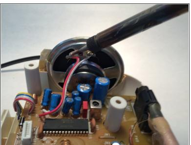
Desolder the wires going to the speaker with a soldering iron.
