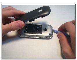
Before completing this step, make sure your device is turned off. Once it is turned off, remove the back cover gently from the phone by prying under the clip near the camera.
