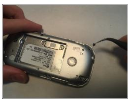
Unscrew the six 2 mm screws from under the back panel.
