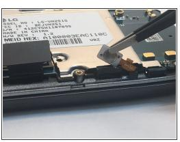
Disconnect volume buttons and camera button from the mounts.
