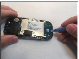
Replace the old motherboard with the new motherboard by reversing previous step, and pressing with plastic tool near ends of board to snap it into place.
