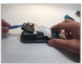
Remove the motherboard from the rest of phone by prying under the board to the side of the headphone jack.
