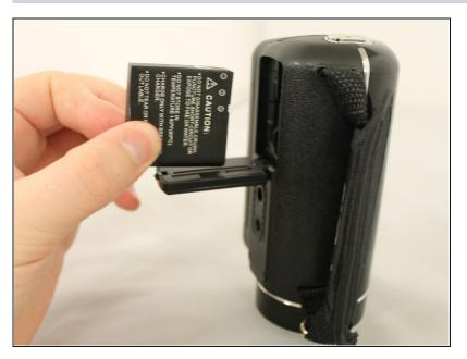
To remove the battery from the device, pull back the tab holding it in place and then remove the battery.
