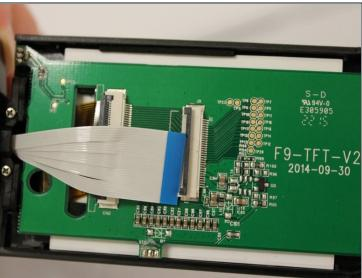
• Use tweezers to open the gray lip of the large white connector and carefully remove it.
