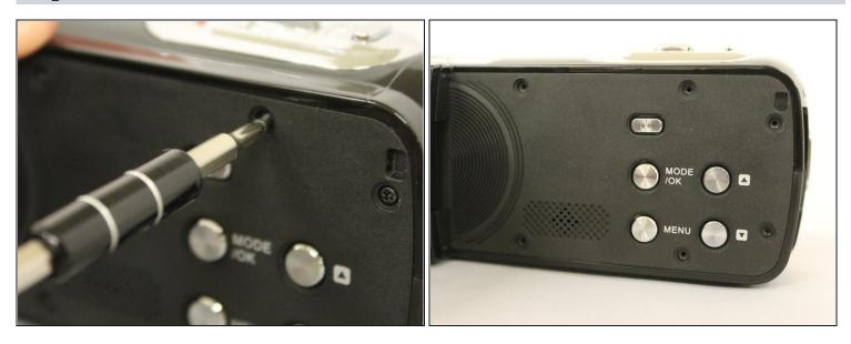
• Use a #00 screwdriver to remove all six 4 mm screws from the side of the device.
