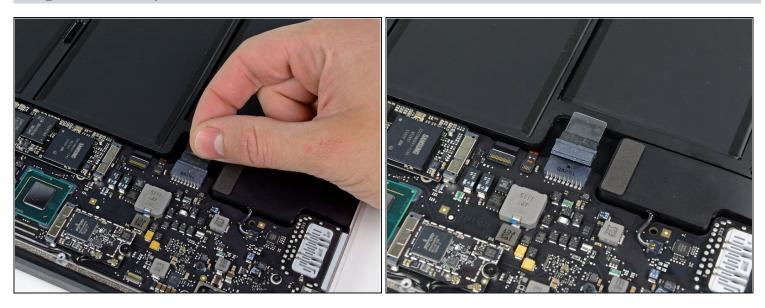
• Grab the clear plastic pull tab attached to the battery connector and pull it toward the front edge of the Air to disconnect the battery from the logic board.
