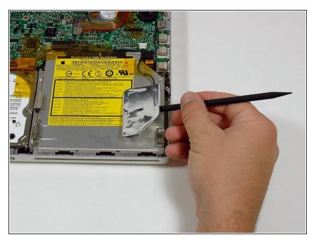
• Use a spudger to pry up the PRAM battery from the optical drive.
