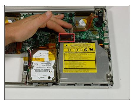
• Disconnect the large black connector from the logic board.
