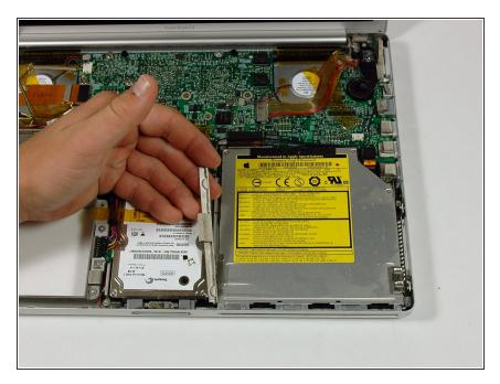
• Remove the retaining bracket.
