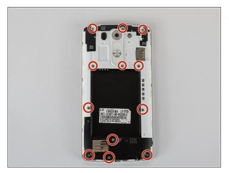
Remove the twelve Phillips #00 screws securing the midframe to the rest of the phone.
