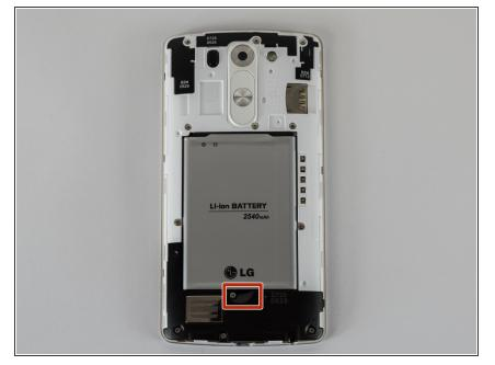
• Remove the battery by lifting from the slot at the bottom of the battery.
