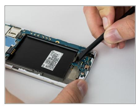
Use the flat edge of a spudger to disconnect the motherboard ribbon connector.
