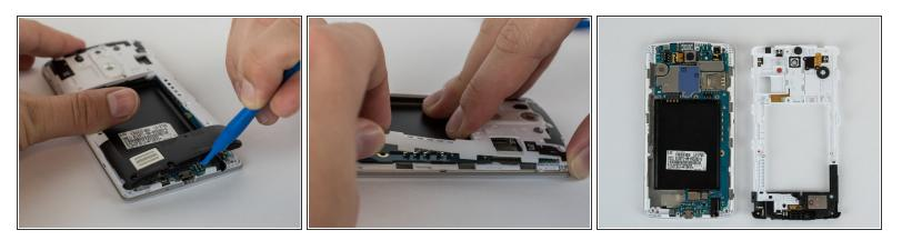
Work a plastic opening tool around the perimeter of the phone to separate the midframe from the rest of the phone.
