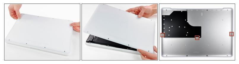
The lower case is constructed of rubber-coated aluminum. Do not excessively bend the aluminum during removal, as any permanent deformation will cause tolerance issues after reassembly.
