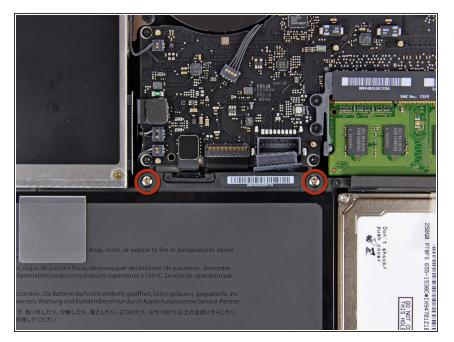
Remove two 5 mm Tri-point screws securing the battery to the upper case.
