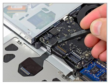
Use the flat end of a spudger to pry the trackpad ribbon cable connector up off the logic board.
