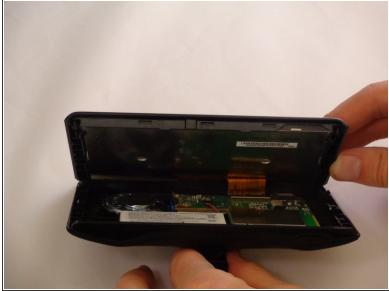
Carefully pull apart the device by opening it up on the opposite side of the nameplate.
