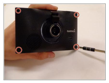
Using a T5 Torx screwdriver, remove four 6 mm screws from the four corners of the back of the device.
