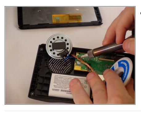
Using a soldering iron, desolder the wire connection between the speaker and the device.
