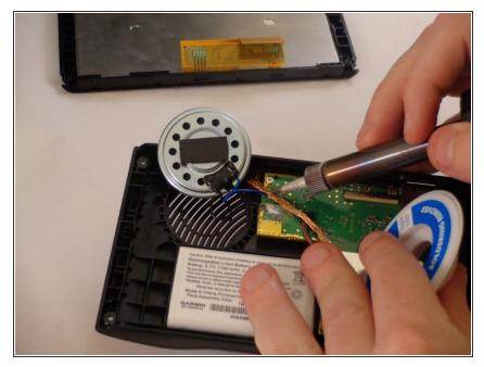
• Using a soldering iron, desolder the wire connection between the speaker and the device.
