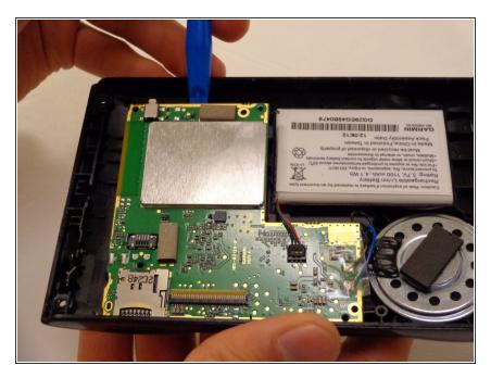
• Using a plastic opening tool, pry the motherboard away from the device.
