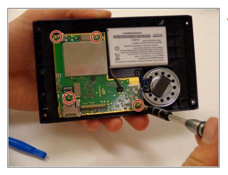
Using a T5 Torx Screwdriver, remove the 5mm screws in the four corners of the motherboard.
