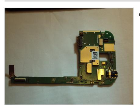
Remove the motherboard from the casing.
