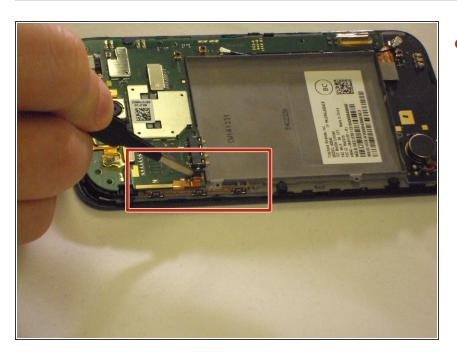
Lift the latch and gently remove the ribbon from the latch.
