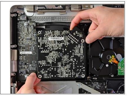
Pull the upper right and lower left corners of the power supply away from the rear case to dislodge the mounting posts attached to the power supply's corners.
