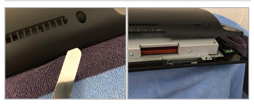
Now carefully pop off the rear plastic cover. Start at the top near the buttons and work toward the bottom.
