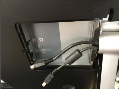
Disconnect the cables on both sides. 4 total.
